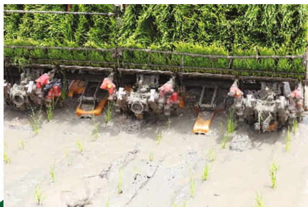
Machine transplanting of rice with mat nursery raised on polythene sheet
