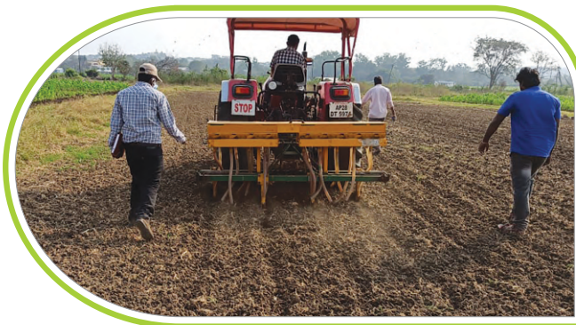
Sowing of cotton with microcontroller based precision planter
