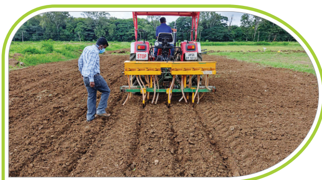
Sowing of maize with microcontroller based precision planter
